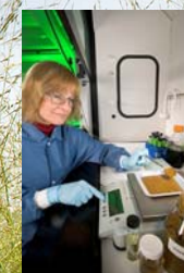
Trap grease sample being prepared for conversion to biodiesel. In the foreground are samples of distilled (left) and crude (center) biodiesel from trap grease.
