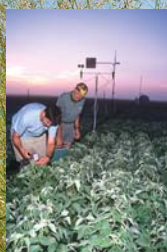
Using a portable photosynthesis analyzer to measure the effects of elevated ozone on growth and development of soybean plants.
